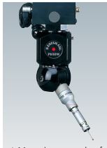
▲ Mounting example of touch-trigger probe
