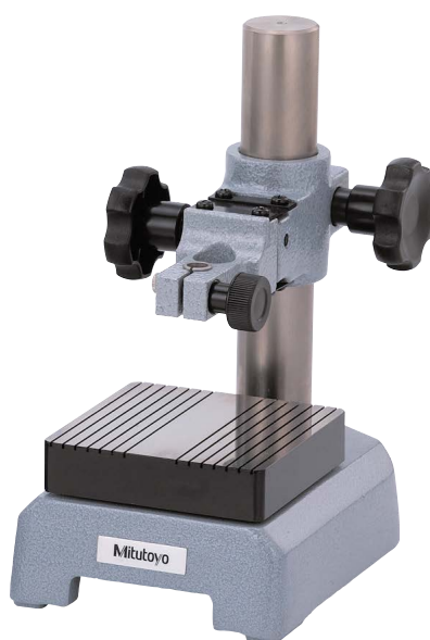
7007-10 (with 90 mm square semi-serrated anvil)
