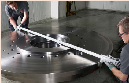
Radiused jaws for accurate ID measurement
